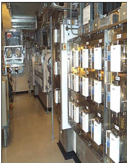
Rod fabrication glovebox Pictures of the Sellafield MOX plant 75, 74
